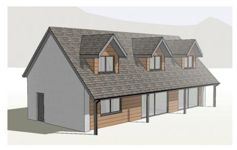
Scottish structural insulated panel experts JML Contracts have brought a series of standardised, low energy structural insulated panel (SIP) designs to the housing market. These off-theshelf homes are intended to provide more affordable low energy housing, incorporating cutting edge technology in ready-made designs.
